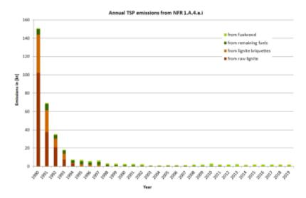
The emission trends for  $PM_{2.5}$ ,  $PM_{10}$ , and TSP are also influenced severely by decreasing coal consumption in small combustion plants, particularly in the period from 1990 to 1994. Since 1995 the emission trend hardly changed. Increasing emissions in the last years are caused by the rising wood combustion.
