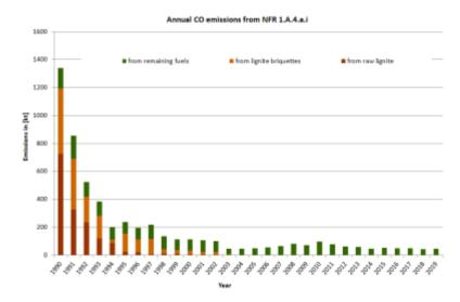
Main driver of the NMVOC and CO emission trends is the decreasing lignite consumption: Since 1990 the fuel use changed from solid fuels causing high NMVOC and CO emissions to gaseous fuels producing much lower emissions.
