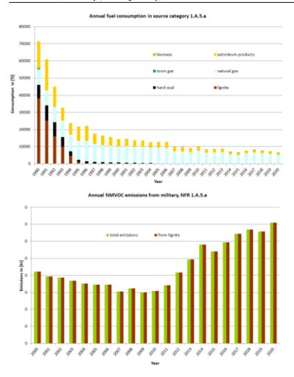
NMVOC emissions show a remarkable falling trend due to the closure of military agencies especially at the beginning of the 1990s as well as the reducing use of lignite for heating purposes.
