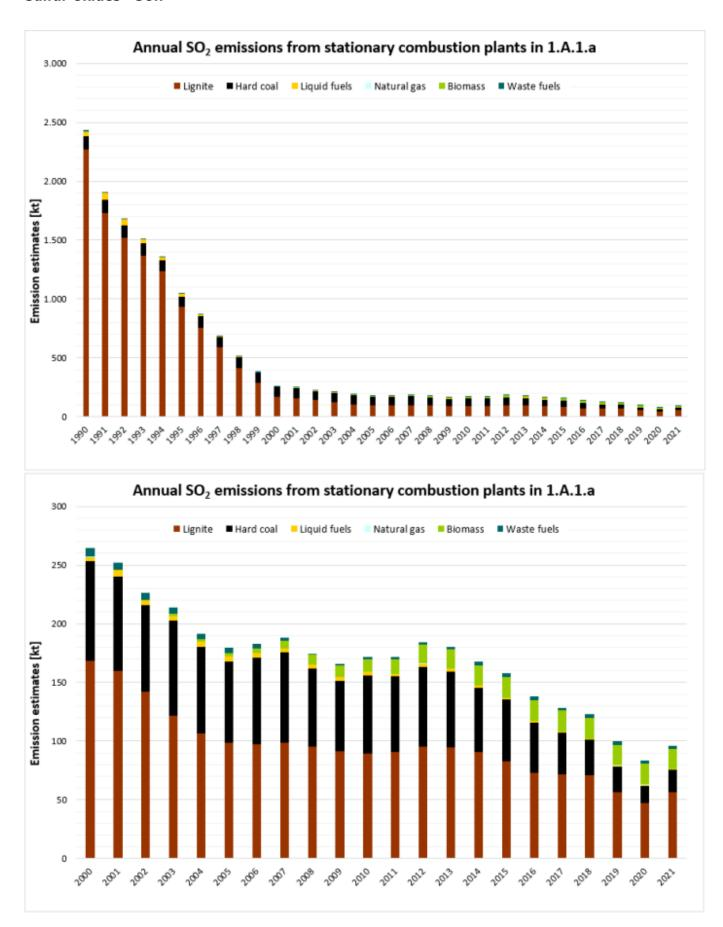
$SO_x$  emission trend shows the big dominance of lignite due to high Sulphur content of lignite fuels. However  $SO_x$  emissions decrease more than lignite consumption does. Before the German Reunification in 1990, lignite fired public power plants in Eastern Germany didn't use flue gas desulphurisation plants. The implementation of stricter regulations in the New German
