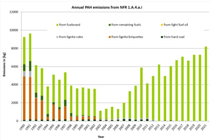
The main driver of the POPs emission trend are coal and fuel-wood. PCDD/F emissions decrease from 1990 to 2003 due to decreasing lignite consumption. The use of firewood and therefore PCDD/F emissions from wood combustion show a constant development.
