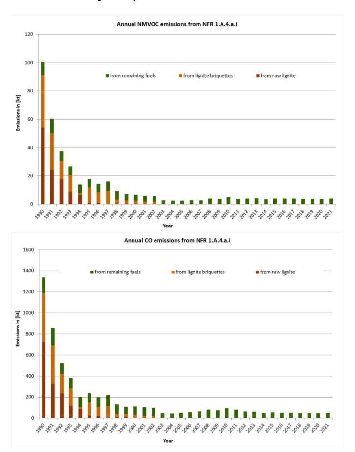
Main driver of the NMVOC and CO emission trends is the decreasing lignite consumption: Since 1990 the fuel use changed from solid fuels causing high NMVOC and CO emissions to gaseous fuels producing much lower emissions.
