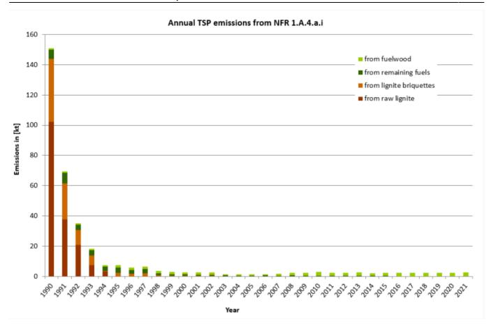
The emission trends for  $PM_{2.5}$ ,  $PM_{10}$ , and TSP are also influenced severely by decreasing coal consumption in small combustion plants, particularly in the period from 1990 to 1994. Since 1995 the emission trend hardly changed. Increasing emissions in the last years are caused by the rising wood combustion.
